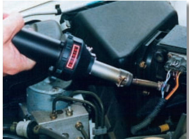
HOT JET S with sieve reflector being used to shrink solder sleeves.
