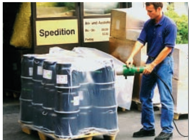
Flamless shrinkwrapping of pallets and bulky items with FORTE S3 for transportation. Working in closed rooms possible.
