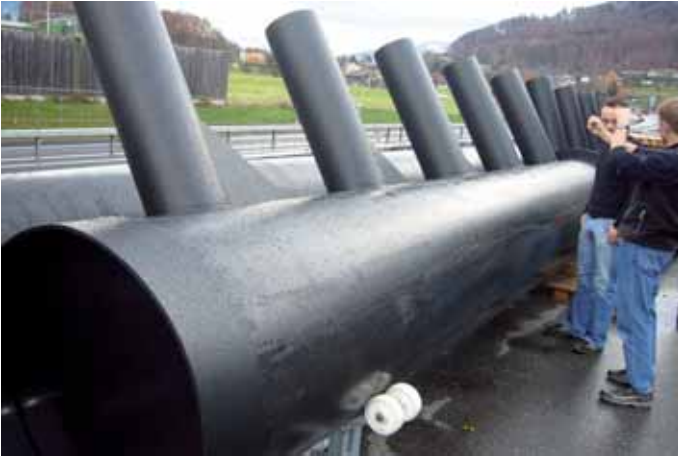
Pipe constructions made of PE for thermal energy systems, Switzerland
