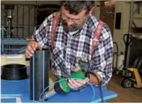
Welding a molded part with TRIAC PID and push-fit speed welding nozzle..
