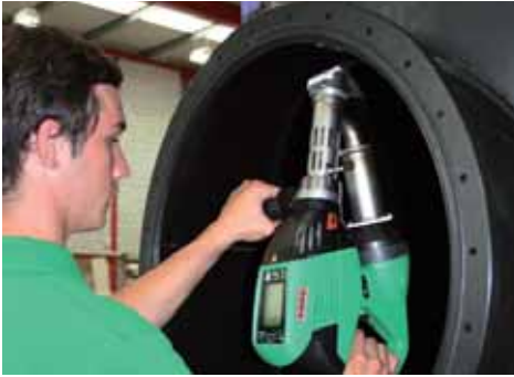
The WELDPLAST S2 also remains easy to handle during vertical welding.
