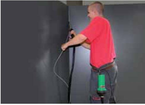
Blower MINOR as air supply for the DIODE PID.
